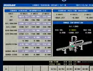
Help setting position of the travel axis of the loader. (Up to 5 different positions can be set and loaded.)
