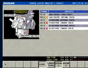
The status of the sensor (swivel unit, turn-over unit) in the loader can be checked in real time.
