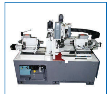
Integrated casting bed
