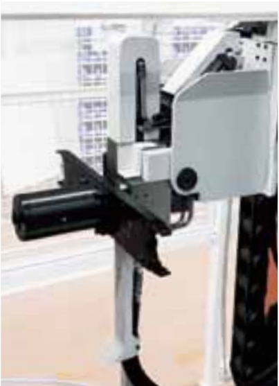
Horizontal ATC operation with a 90° head attach mounted.
