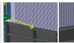
Coolant flushing at base of X axis chip cover
