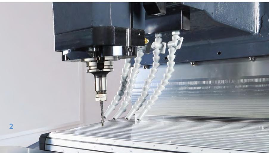
Dual pallet was applied to improve productivity, and a thermal displacement compensation program was applied as standard for precise and fast processing of various parts. In addition, it provides various convenient functions such as EZ work.
