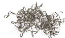
Cutting chip when not in use with vibration cutting control function
